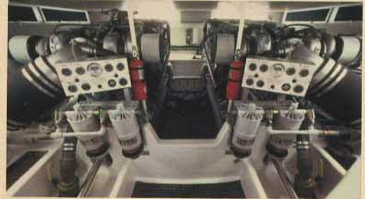
VIKING MOUNTS THESE 12-CYLINDER TURBODIESELS ON SOLID STEEL BEAMS.
